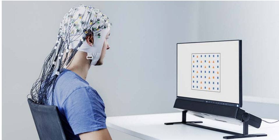
Figure 6 A volunteer wearing an EEG cap in front to the Tobii Pro Spectrum eye tracking platform. Image reproduced with permission of Acuity ETS Ltd., Reading, UK.
